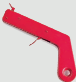
Ignition Gun Used for igniting the ignition powder. Accepts regular lighter flints as a replacement. deignición.
