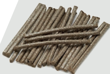
Sealing Rod. Strands of refractory paste used to prevent loss of molten copper between the mold walls and the conductors to be welded.
