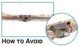
Use the appropriate clamp for each type of mold and verify that it is fully closed and secured before starting the welding process. A secure closure with the correct clamp will prevent material leaks and ensure a high-quality weld.
