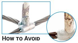
It is very important to correctly place a single disc inside the chamber before pouring the aluminothermic powder. Verify that the disc is positioned as indicated in the instructions, and only one unit is used to ensure a proper metal flow and prevent blockage of the welding channel.
