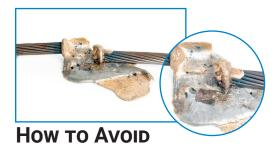
In some types of connections, applying sealing paste is the only way to ensure a perfect connection. This measure prevents leaks and compression loss in the exothermic process, while also protecting the weld from corrosion, extending its lifespan, and maintaining the system's safety in optimal conditions.
