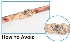
Moisture is one of the main enemies of exothermic welding. It can create bubbles in the joint, weakening the structure and affecting its conductivity. Before starting, ensure all components are dry. This step can prevent many long-term issues.
