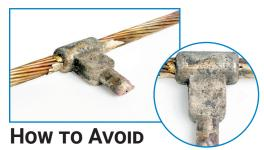
Ensure you use the specific cartridge for each type of weld. Verifying its compatibility with **the KLK AppWeld application** and confirming the weld size will prevent issues with weak or faulty connections.
